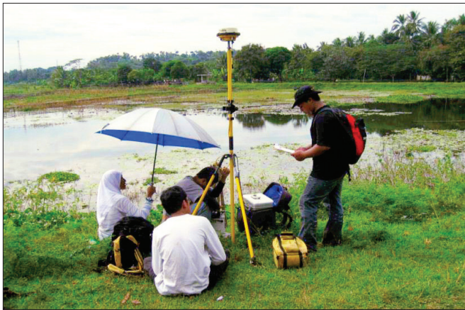
Operating a La Coste-Romberg meter to obtain gravity data at the Gadjadara University Geophysics Expedition (Indonesia) 2009.
