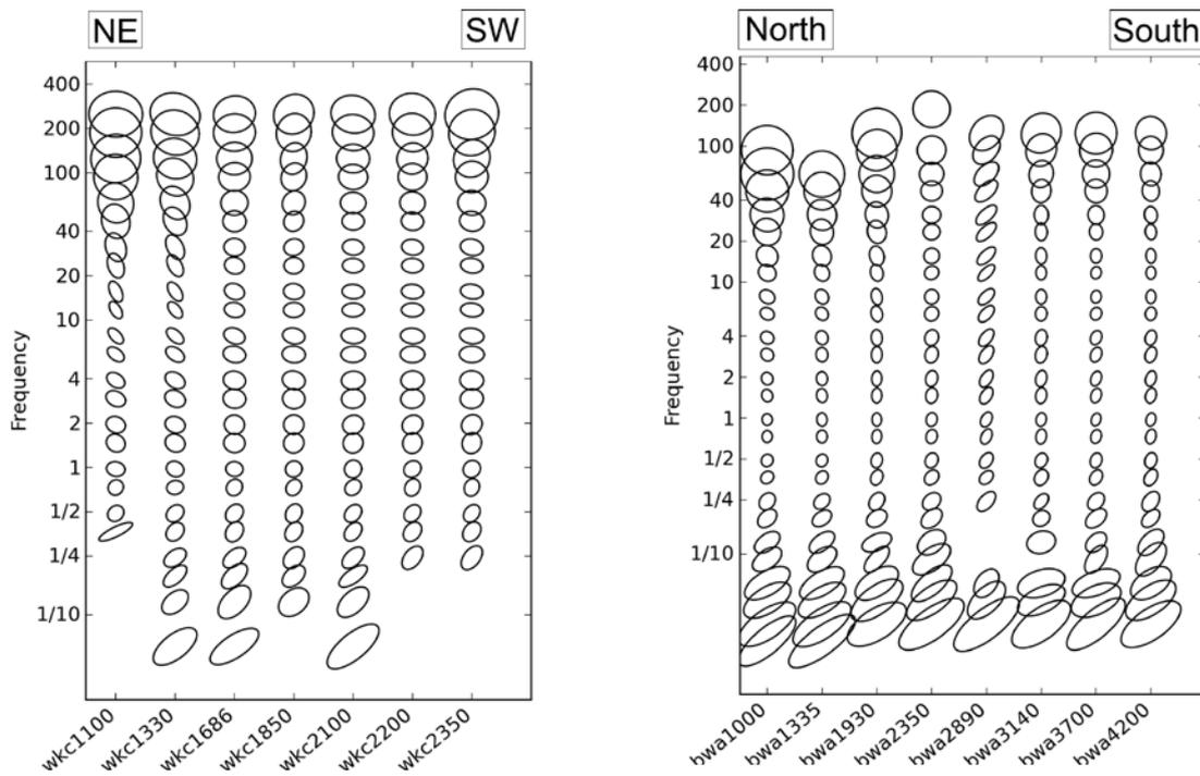
Figure 2. Phase tensor ellipse pseudosections along a) Line C at Wabma Kadarbu; and b) Line A at Beresford Spring. Note the difference in response at 20 Hz between Blanches Cup Spring (located at station WKC2350) in a), and the Beresford Spring (located at BWA2890) in b).
