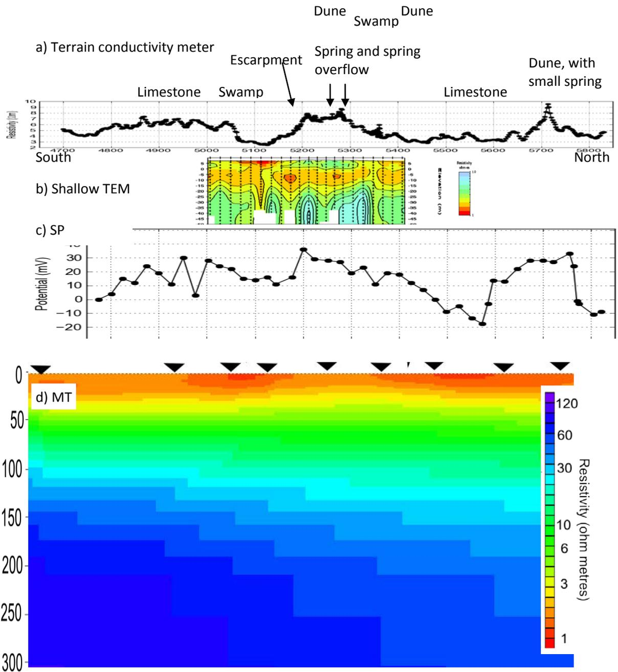
Figure 1. Comparison plot for data sets collected at Line A, Wabma Kadarbu. A) terrain conductivity data; b) shallow TEM data; c) SP data and d) MT resistivity data. On d) triangles indicate locations of MT measurement sites.
